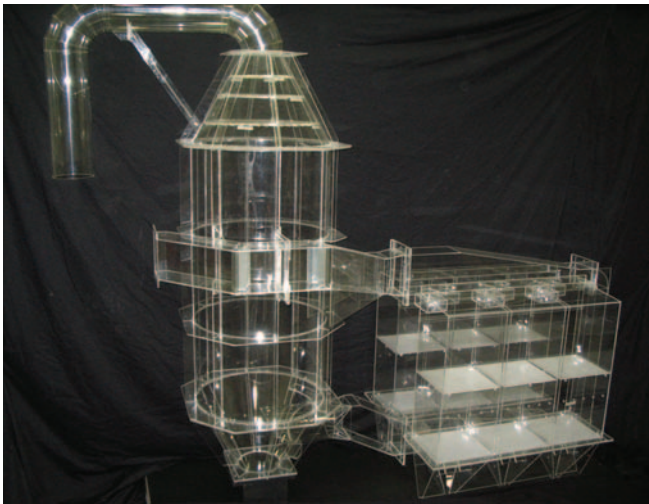
Figure 8: Typical baghouse model
