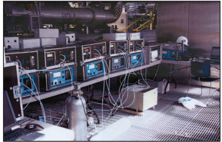
Figure 1: AIG tuning using an ECOS setup with 7 NO/O 2 analyzers in parallel
