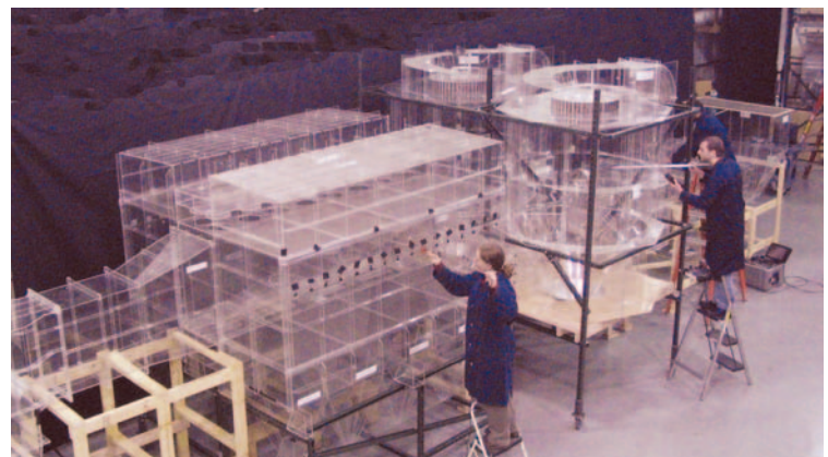
Figure 6: Physical flow model of a power plant dry scrubber and baghouse
