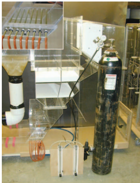
Figure 13: Physical model testing of thermal mixing via tracer gas injection (SCR economizer bypass)
