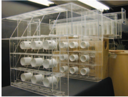
Figure 9: CFD and physical model of a windbox
