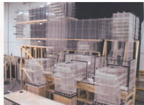
Figure 8: Comparison of CFD and physical model results for an FGD duct system where flow from 3 units (1,750 MW total) combine to feed 3 new booster fans (CFD pressure drop 1.19 "H 2 O; Physical pressure drop 1.27 "H 2 O)
