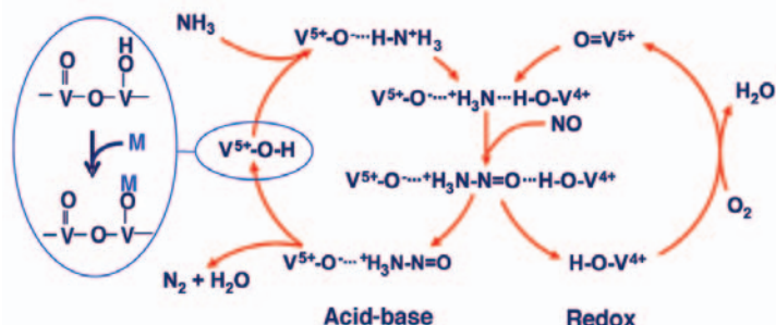
Figure 9: Basically, the SCR reaction involves both acid-base and redox catalytic functions. The reaction is initiated by the adsorption of ammonia on Brønsted acid sites ( V^{5+}\text{-OH} ), followed by “activation” of ammonia via reaction with redox sites ( V=O ). This “activated” form of ammonia then reacts with gaseous or weakly adsorbed \text{NO} , producing \text{N}_2 and \text{H}_2\text{O} while releasing V^{4+}\text{-OH} . To complete the catalytic cycle, the V^{4+}\text{-OH} species is oxidized by either \text{NO} or \text{O}_2 to regenerate the original V=O species (from [1])
