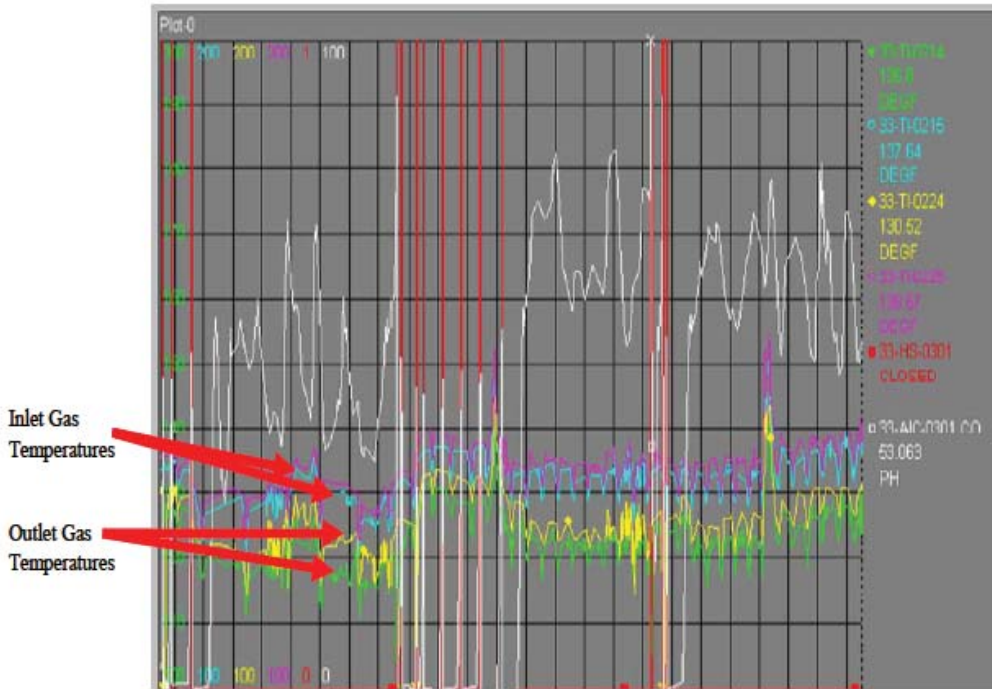
Figure 13: 24-hour PI chart of two-module membrane WESP at SSCC, Stevenson, AL
