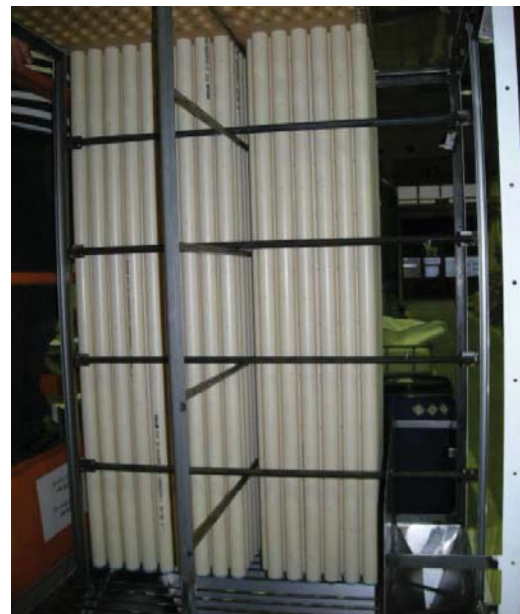
Figure 19: Physical flow model with perforated plastic tubes
