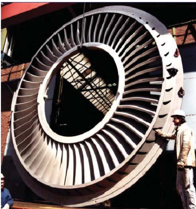
Figure 6 – LP Last Stage Stationary Blade Ring with Forward Leaning Design
