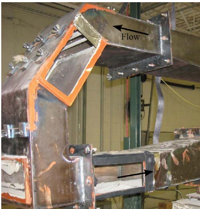
Figure 7: Physical model with clear windows for viewing ash flow during Hot Wind Tunnel operation
