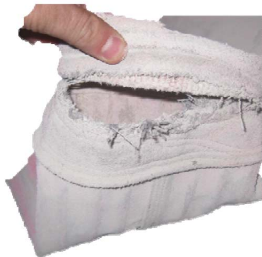
FIGURE 26: Failure at top snap band cuff
