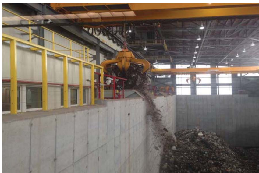
FIGURE 29: Automated refuse crane technology.
