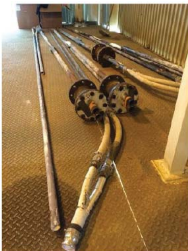
Fig 24: Each port had two lances, a short (~6 ft.) and long (~13 ft) lance
