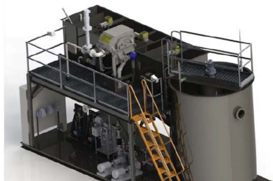
Figure 25: CoMag Ballasted Flocculation Clarifier Skid.
