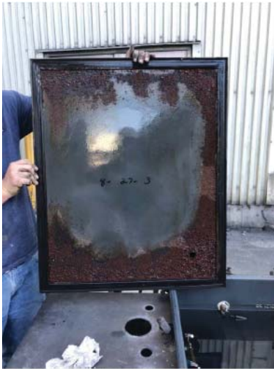
Figure 28: Internal T/R corrosion indicating oxygen in the T/R
