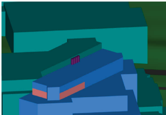
Figure 4: Research building roof and exhaust stack geometry (Building intake louvers in orange)
