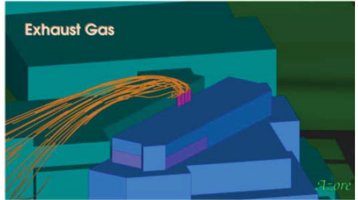
(a) (b) Figure 9: Streamline plots of (a) ambient wind and (b) exhaust gas
