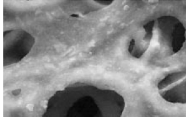
Coated Polyester Felt at 1000x Large pores allow submicron dust to pass through
