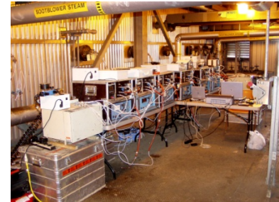
Multi-point NO x /O 2 Analyzer Set-up
