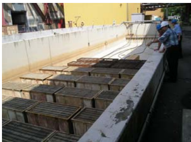
Rejuvenation Tank During Catalyst Loading
