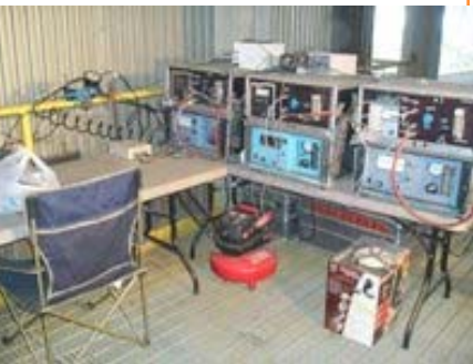
Multi-point NO x /O 2 Instrumentation Set-up
